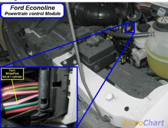
The PCM is under the hood, next to the brake master cylinder.
